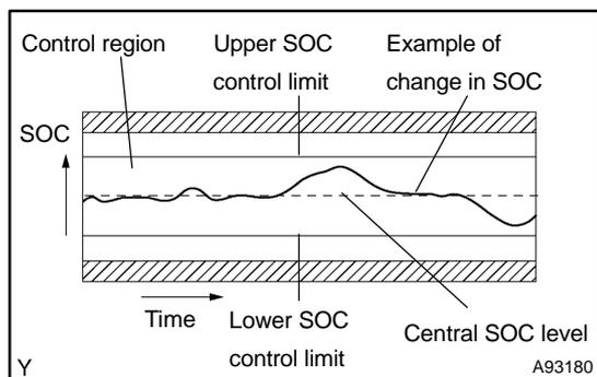
The battery ECU calculates the SOC (state of charge) of the HV battery by estimating the amperage that flows into the HV battery and monitoring other values.
